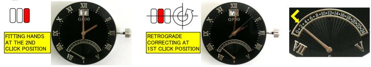
5) PULL THE CROWN TO 2ND CLICK POSITION AND TURN THE HAND. THE INDICATION GAP BETWEEN MIN HAND AND RETROGRADE HAND SHOULD BE WITHIN +/-15 MINUTES. CHECK THE TIME (WITHIN +/- 40min of 2:00 A.M.) WHEN THE DATE IS FULLY CHANGED.
