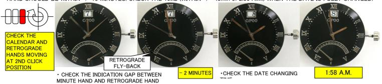
CAUTION: TURNING HAND (ANTI-CLOCKWISE) AT 2ND CLICK POSITION WHEN RETROGRADE HAND IS AT 0 POINT POSITION WILL CAUSE DIFFERENT TIME-LAG BETWEEN CENTRE TIME AND RETROGRADE HAND TIME.
